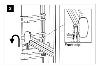
2. Locate the front clip onto the shelf runner and firmly push the front of the guide down until the front clip is secured into place.
