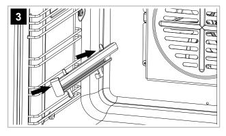
1 Note: The Telescopic guides can only be attached to the top part of the top, middle and bottom sections of the shelves as shown below.
