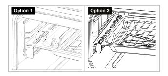
Note: Please ensure the wires / oven pan locate around the small tabs on the telescopic runner.
