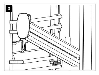
The Telescopic guide should now be fitted correctly and secure to the shelf runner.
