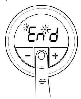
Press the function button until 'end' appears on the display
