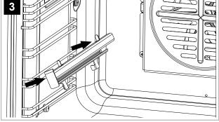
Note: The Telescopic guides can only be attached to the top part of the top, middle and bottom sections of the shelves as shown below.
