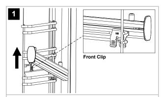
Push the front of the guide upwards firmly, ensuring the front clip is released from the shelf runner.
