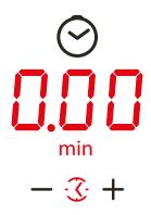
Before activating a timer the control has to be switched on. Switching the control off deactivates cooking zone related timers. The egg timer stays active after switching the control off.
