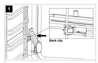
1. Secure the back clip in between the shelf runner. Ensure the guide is fully pushed back towards the back of shelf runner.
