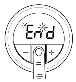
Press the function button until 'end' appears on the display
