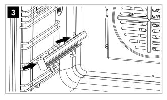
Note: The Telescopic guides can only be attached to the top part of the top, middle and bottom sections of the shelves as shown below.
