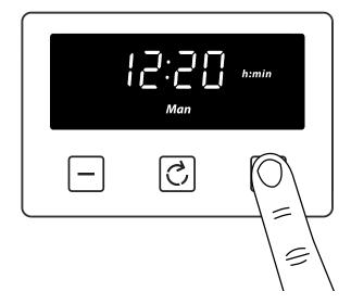
1. Press and hold the plus button for 3-5 seconds
