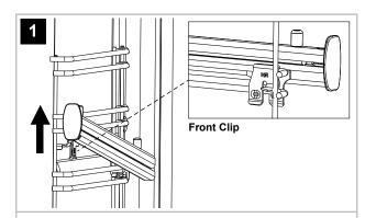
1. Push the front of the guide upwards firmly, ensuring the front clip is released from the shelf runner.
