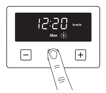
To switch off, press and hold the menu button for 2 seconds. The connectivity symbol will disappear
