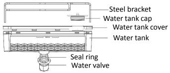
2. Remove the large cover, then fill the water directly.
