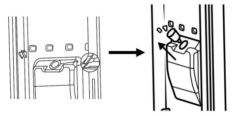
Clean all parts (water tank and cover, seal ring and water valve with hot soapy water, then rinse thoroughly and dry.
