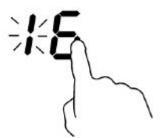
While the units digit is flashing, use the touch control slider to set the units digit of the cooking duration time (between 0 and 9).
