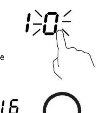
4. Touch the timer control again. The units digit is accepted and the tens digit starts flashing.
