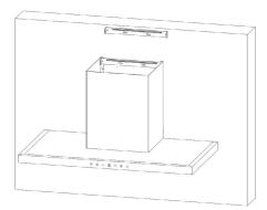
6) Pull out the telescopic upper chimney section to the relevant height required to reach the ceiling and to be aligned with the upper chimney support bracket. Use the 2 x ST4.2\*9.5 screws to secure the upper chimney section to the upper chimney support bracket to secure it in place.
