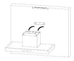
3) Use the 2 x M5\*12 screws to secure the body of the hood to the hood body support bracket. Now attach the 150mm diameter ducting pipe (which is not included with the hood, but is available as an optional extra) to the air outlet collar on top of the motor and secure it with a jubilee clip.
