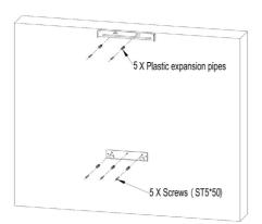
2) Locate the holes on the rear of the hood body with the lugs on the hood body support bracket to hang the hood body on the wall.
