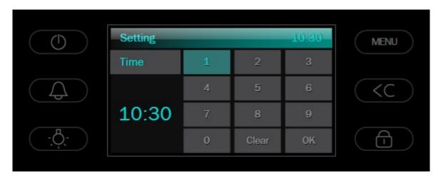
You can display the clock in either 12 hour or 24 hour format. From the main menu, select 'settings' and then 'clock format'. Touch either '12 hour' or '24 hour' and touch 'OK' to confirm.
