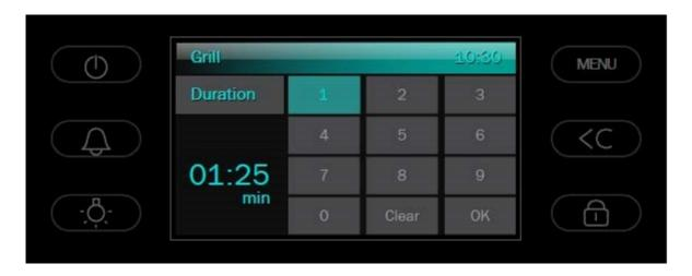
If you want cooking to start immediately and don't require cooking to start and finish automatically later on, then you don't need to set a start time or finish time at this stage. Simply touch 'OK' and cooking will start immediately.
