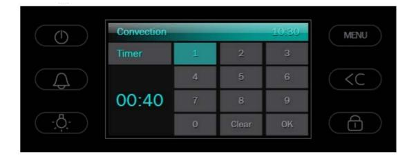
When the minute minder duration time has elapsed the buzzer will sound. Touch the minute minder bell key  $\triangle$  to silence the buzzer.
