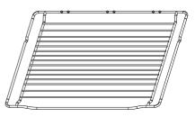
Shelf support rails: Used to support the wire shelf and grill pan if required. These shelf support rails on the right and left sides of the oven can be removed.
