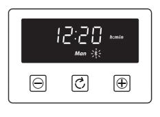
Press and hold the function key for 5 seconds to deactivate the bluetooth connectivity function. The connectivity symbol will disappear.
