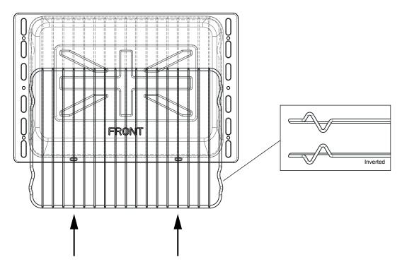
For the quickest toasting results, always place the shelf into the top position runners and place the grill pan with the trivet on the shelf.
