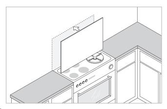
Firstly offer up the back of the Splashback to the worktop /wall to check the fit. Use the spacers provided to achieve a good fit. <u>There needs to be a gap of 2-3 mm around all</u> 4 sides.
