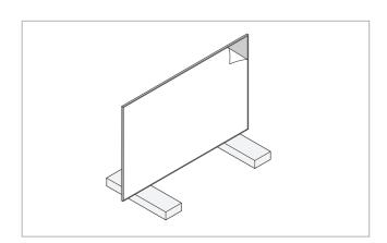
Take the Splashback away from the wall making sure to keep all corners safe from hard surfaces. Remove the covering from the self adhesive backing.
