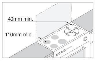
Firstly check the dimensions. The minimum distance from the rear of the hob should be no less than 40mm or 110mm to a heat source dependant on the installation.
