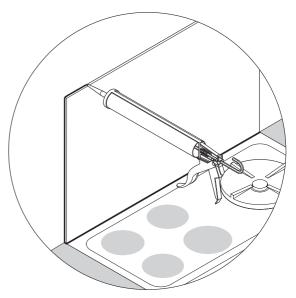
**6** The 4 exposed edges of the Splashback must be sealed with a bead of silicone sealant no less than 2-3 mm in thickness.
