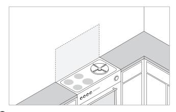
Ensure that the wall being fixed to is completely flat, non porous, dry, dust and grease free. Any gap between the worktop and the wall must be sealed to exclude moisture. PLEASE NOTE: This product should not be fitted over any existing tiling or splashbacks.
