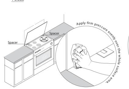
Place the bottom edge of the splashback to the back lip of the worktop / wall on the spacers provided then push the splashback to the wall and apply firm pressure evenly over the whole surface area. Please note once the adhesive has made contact with the wall you will not be able to adjust or remove. Please take extra care when fitting. Ensure that the 3mm spacers are left while the sealant bonds to the wall. Finally after 2-3 hours remove the spacers.
