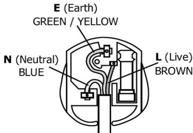
be connected to the terminal marked L (Live), or coloured Red.
