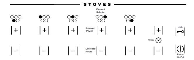
When the hob is first switched the controller will illuminate parts of its displays, accompanied by a beep. This is the controller testing and calibrating itself. When this process is complete the neon adjacent to the lock pad will light, to indicate the hob is ready for use but locked for safety.
