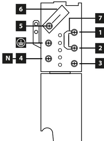
**Note;** Ensure Link screw connections are tight!
