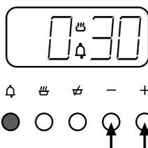
Press the minute minder button, then use the plus and minus buttons to set the required time.
