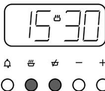
To set the programmer to manual operation at any time (cancelling any automatic setting), press the cook time and ready time buttons simultaneously. The programmer must be set to manual before the appliance can be used manually.
