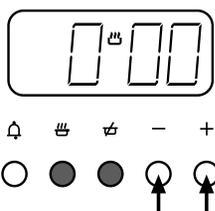
Press the cook time and ready time buttons simultaneously, and keep the buttons depressed. Use the plus and minus buttons to set the time of day, eg; 12.00.
