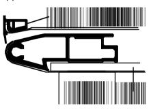
When securing the appliance, the fixing screws provided are driven through the edging strips into the cabinet - the seal will straighten up and sit flush to the cabinet when the screws are fully home.
