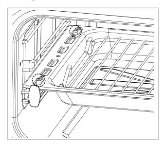
Note: Please ensure the wires / oven pan locate around the small tabs on the telescopic runner.
