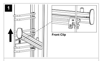
1. Push the front of the runner upwards firmly, ensuring the front clip is released from the shelf guide.
