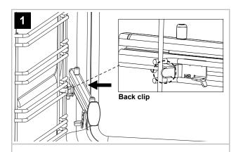
1. Secure the back clip in between the shelf guide. Ensure the runner is fully pushed back towards the back of shelf guide.
