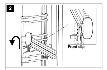
2. Locate the front clip onto the shelf guide and firmly push the front of the runner down until the front clip is secured into place.
