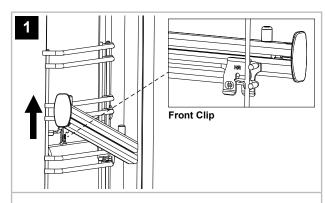
1. Push the front of the runner upwards firmly, ensuring the front clip is released from the shelf guide.
