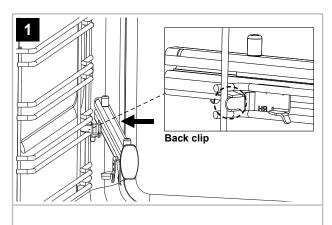
Secure the back clip in between the shelf guide. Ensure the runner is fully pushed back towards the back of shelf guide.
