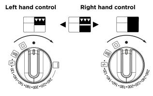
With the upper oven activated, by turning the right hand control knob to a function or temperature, the lower oven can operate. The lower oven cannot be used separately.
