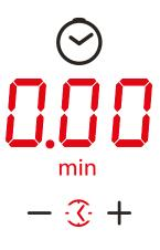
Before activating a timer the control has to be switched on. Switching the control off deactivates cooking zone related timers. The egg timer stays active after switching the control off.
