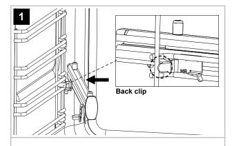
Secure the back clip in between the shelf guide. Ensure the runner is fully pushed back towards the back of shelf guide.
