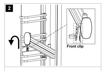
2. Locate the front clip onto the shelf guide and firmly push the front of the runner down until the front clip is secured into place.
