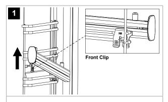
Push the front of the runner upwards firmly, ensuring the front clip is released from the shelf guide.
