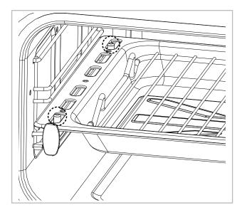
• Note: Please ensure the wires / oven pan locate around the small tabs on the telescopic runner.
