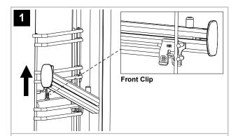
Push the front of the runner upwards firmly, ensuring the front clip is released from the shelf guide.
