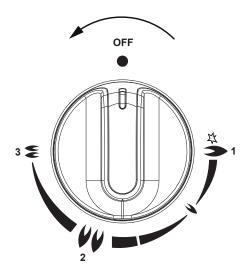
To ignite the outer burner of the wok, turn the control knob to the ignition and flame symbol (1). Hold for 15 seconds until the flame takes hold. Then turn the control knob to the desired power.
