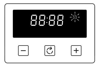
Once the Key lock is active, the buttons will be inactive. A two beep signal will be heard if the buttons are pressed.
