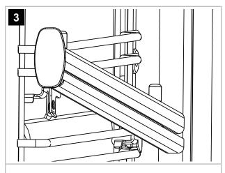
The Telescopic guide should now be fitted correctly and secure to the shelf runner.
