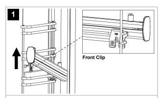
Push the front of the guide upwards firmly, ensuring the front clip is released from the shelf runner.
