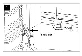
Secure the back clip in between the shelf runner. Ensure the guide is fully pushed back towards the back of shelf runner.
