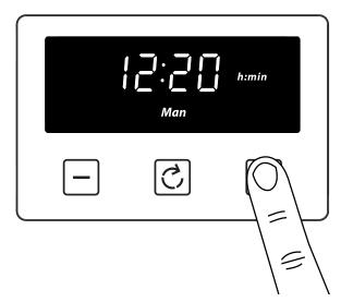
1. Press and hold the plus button for 3–5 seconds
