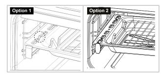
Note: Please ensure the wires / oven pan locate around the small tabs on the telescopic runner.
