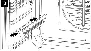
Note: The Telescopic guides can only be attached to the top part of the top, middle and bottom sections of the shelves as shown below.
