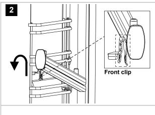
2. Locate the front clip onto the shelf runner and firmly push the front of the guide down until the front clip is secured into place.
